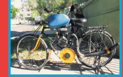
Top to bottom: 'Rikimbili' bicycle propelled by a fumigation machine engine, Havana (2003); by a water pump engine (2005); and by a military tank engine (2005).
